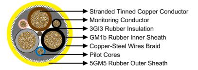
Conductors: Flexible stranded tinned copper conductor.
